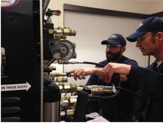
Students operate the \$33,000 hydraulics training board. There are 18 different hydraulic circuits that they set up and operate, taking pressure and flow readings at different stages of circuit function.
